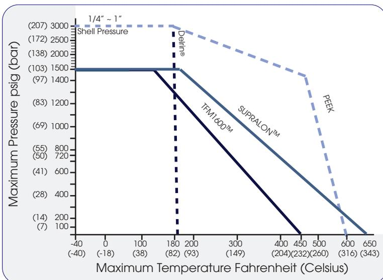
Note: Maximum pressure & temperature is limited to the seat material rating
