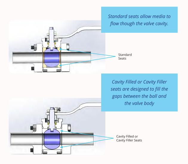
Note: Each application has different requirements and may use the standard or the cavity filled seats. For example, ASME – BPE prefers utilizing standard seats over cavity filled for pharmaceutical applications, while most Food and Beverage applications require cavity filled seats.
